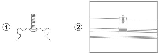
2) Place the lamp in an appropriate position on the mesh cover of the reptile terrarium, and install the gasket, butterfly nut, and nut cover on the bolt in turn.
