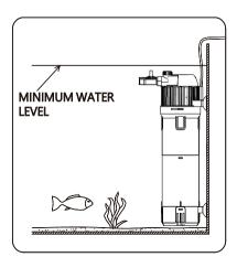
Reminder: Make sure the filter is positioned above the minimum water level.
