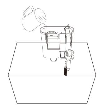
2) Be sure the water level in the tank is not lower than the water mark.
