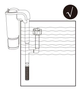
3. Do not use a tank with a depth below 9.6inches to avoid oil remover failure.
