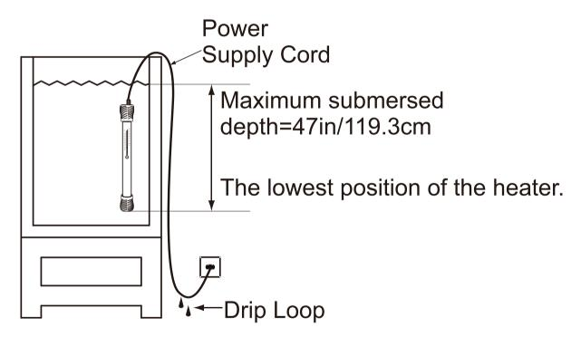
1.To avoid the possibility of the appliance plug or outlet getting wet, position aquarium stand and tank to one side of a wall-mounted outlet to prevent water from dripping onto the outlet or plug. A drip loop, shown in the figure above, should be arranged by the user for each cord.
