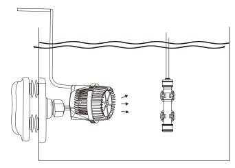
Place the hygger heater fully submersible when it's on, unplug it and wait for 15 minutes before changing the water or removing the heater.
